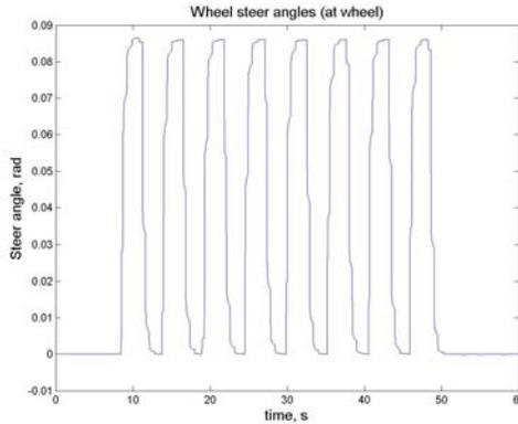
Figure 8: Front wheels steer angle from lateral driver model
