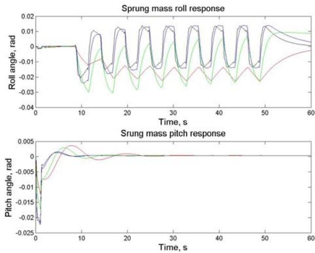
Figure 4: Vehicle sprung mass roll and pitch responses
