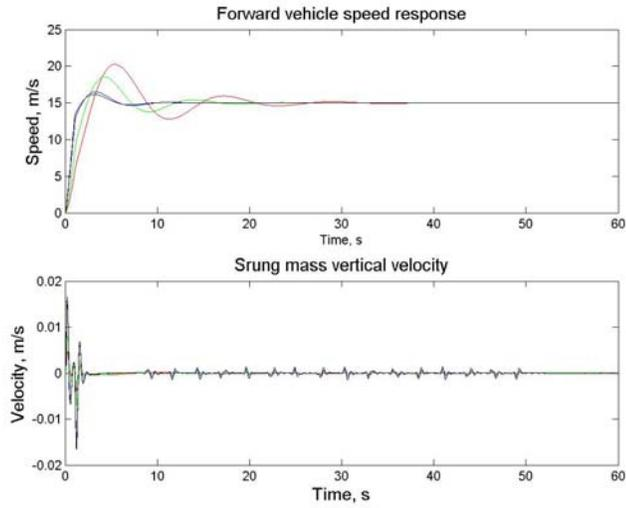
Figure 5: Vehicle forward speed and sprung mass vertical displacement responses
