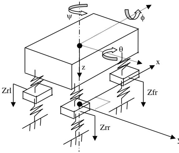
Figure 1: Vehicle local coordinate system and sign convention
