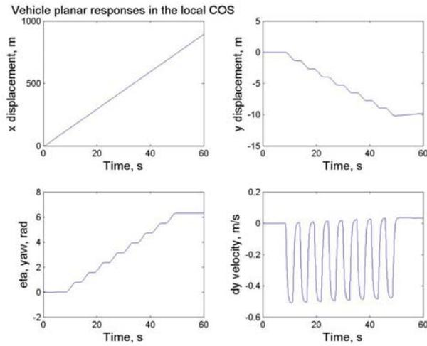
Figure 6: Vehicle yaw and planar response in the local reference frame
