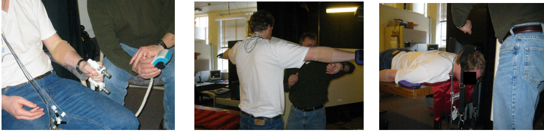
Figure 2a. Hand dynamometer used for finger flexors calibration contractions; Figure 2b. Trapezius calibration contractions and hand weights; Figure 2c. Mid-cervical extensor calibration contraction measured in prone position.
