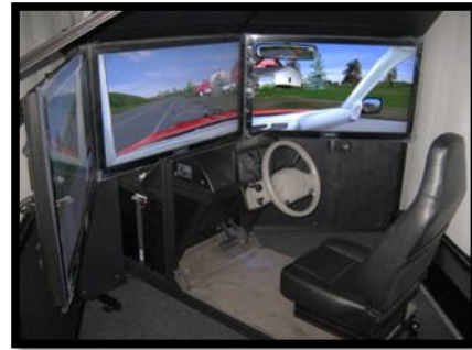
Figure 1 Three Screen Quarter Cab MiniSim
