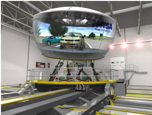
Figure 2 Computer-generated image of a NADS cab inside the NADS dome during a driving maneuver.
