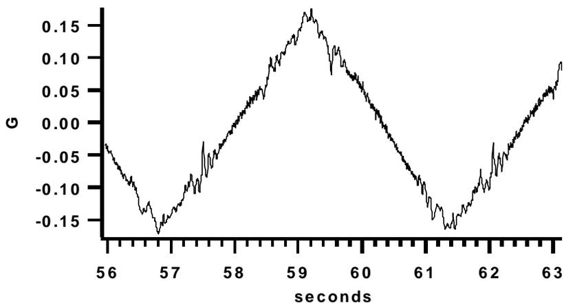
FIGURE 10 X-acceleration Response, 0.1Hz, 1.4 m/s<sup>2</sup>
