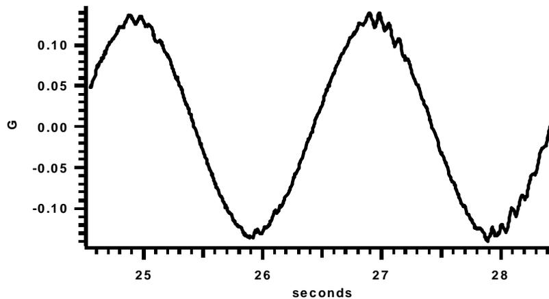
**FIGURE 3 X response to 1/2 Hz 1.28 m/s<sup>2</sup> input.**
