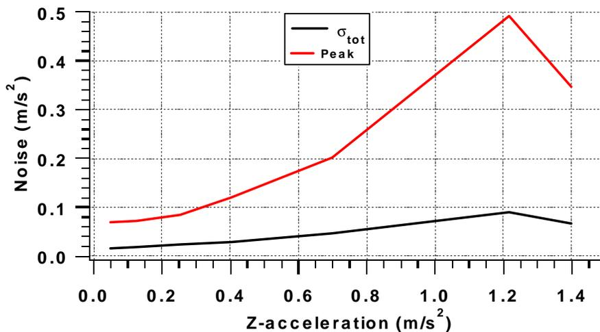
FIGURE 7 Y-noise for 0.5Hz Z-acceleration.
