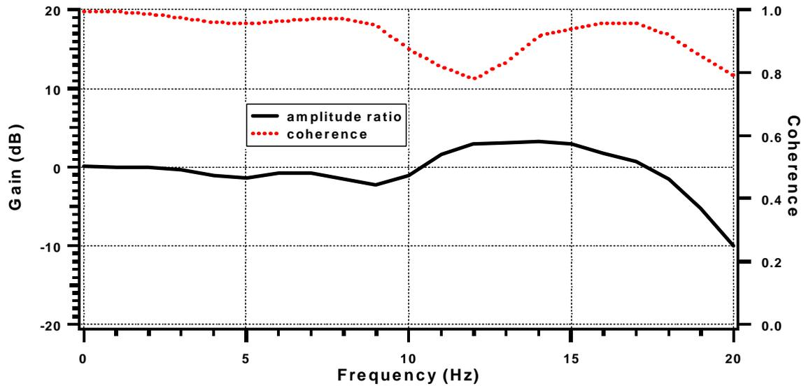
FIGURE 1a X-Transfer Function Amplitude Ratio and Coherence.
