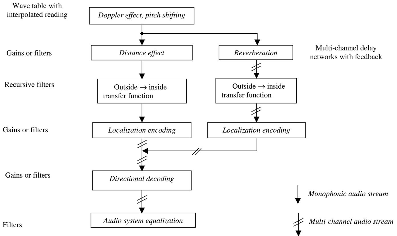
Figure 4: General architecture of sound processing
