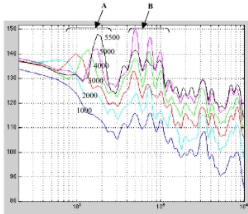
Figure 11 : cumulated spectra for the various RPMs as recorder by the accelerometer.
