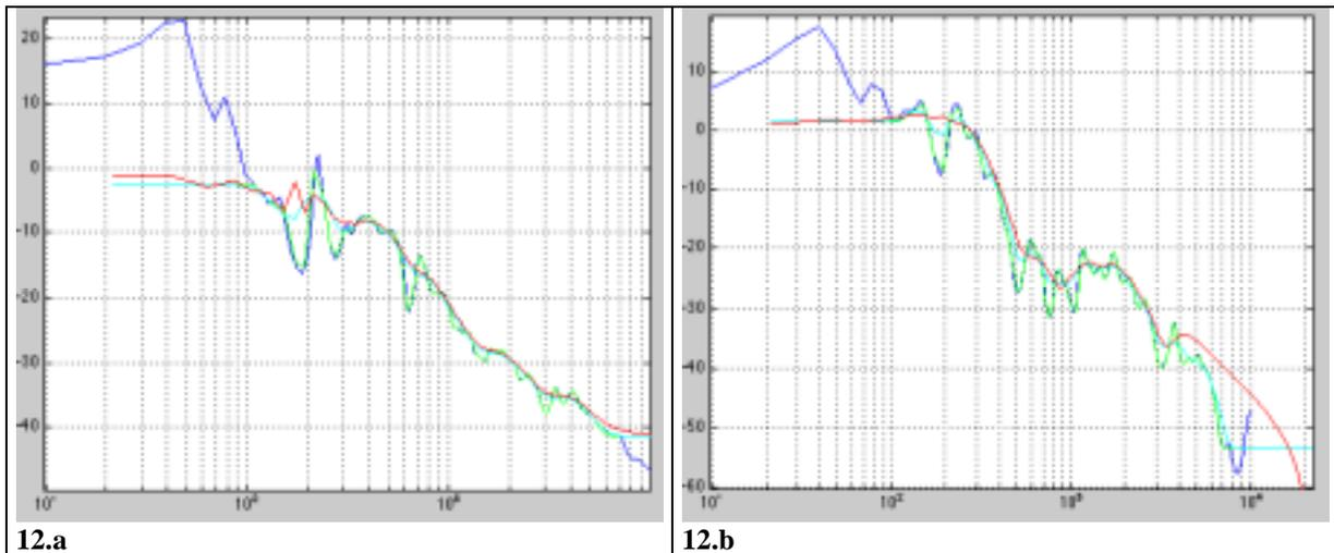
Figure 12: Corrective filters, cabin/exterior. 12.a aerial microphone. 12.b Accelerometer microphone. Direct transfer function (blue), limited in frequency (green), smoothed (cyan), estimated with a 12<sup>th</sup> order ARMA filter (red).
