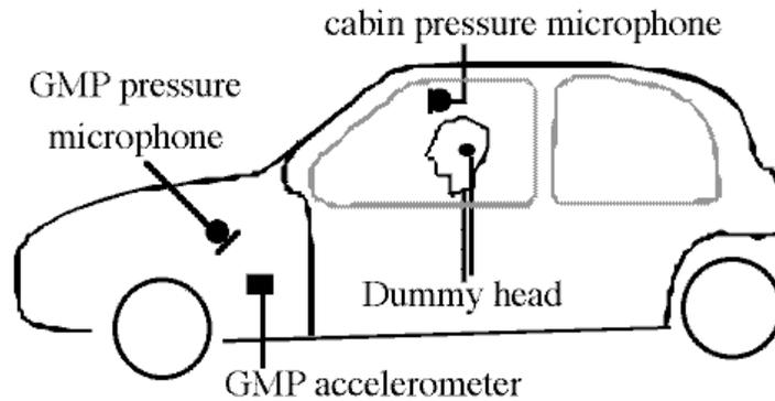
figure 8: Localization of the sensors used for engine noise measurement : cabin microphone (B&K 4165 1/2 inches), dummy head (HEAD ACOUSTICS HMS II), GMP microphone (B&K 4165), and GMP accelerometer
