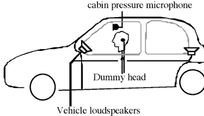
figure 9: Localization of the sensors used for audio system characterization.
