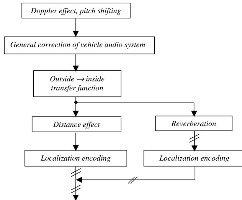
Figure 5: General architecture of sound sources processing, with vehicle equalization module moved upstream of the 3D sound processing
