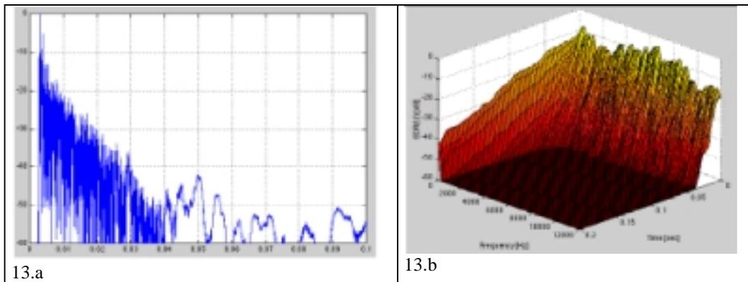
*figure 13: 13.a loudspeaker echogram. 13.b time vs. frequency distribution associated to impulse response*
