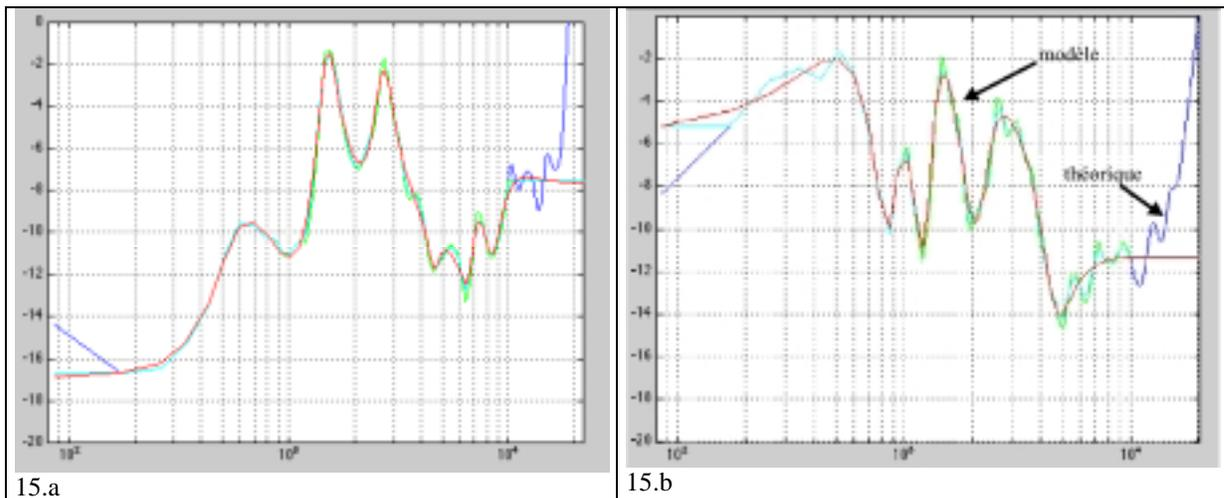
figure 15: correction filter magnitude derived from the global (15.a) or diffuse (15.b) field spectral characterization. Direct transfer function (blue), limited in frequency (green), smoothed (cyan), estimated with a 12<sup>th</sup> order ARMA filter (red)
