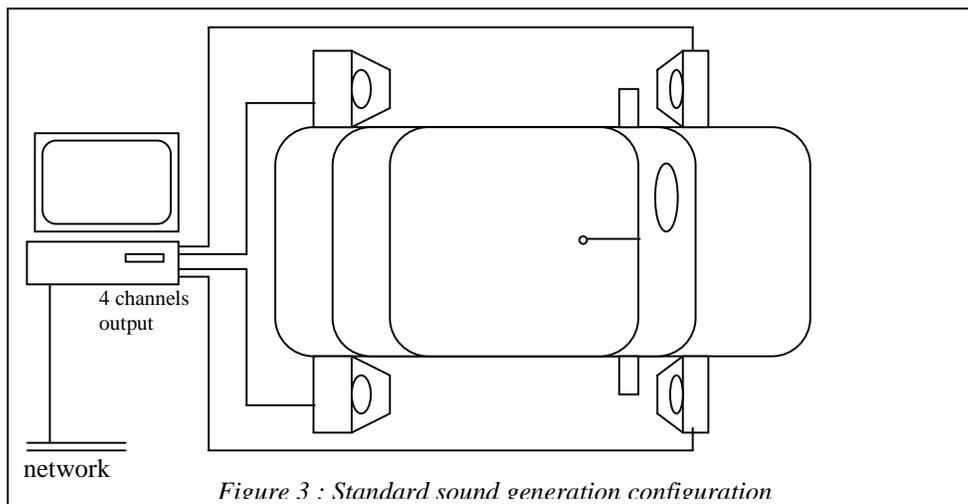
However, this configuration suffers from losses in power transmission, as the sounds are generated in an open space, often forcing the driver to open the windows of the cockpit to have a better perception of the sound environment, losing part of the filtering effect of the cockpit and the balance between the channels that generate the 3D effect.
