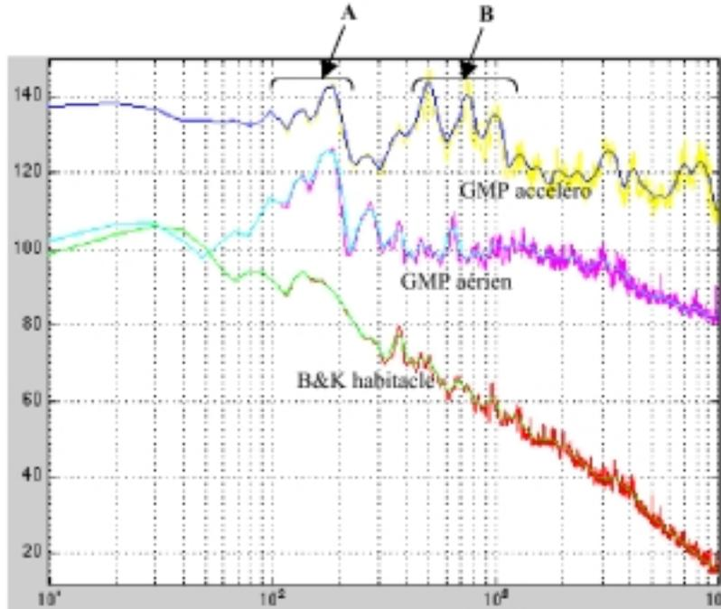
Figure 10 : cumulated and averaged spectra on the various engine RPMs, as measured by the accelerometer (blue), aerial microphone (cyan) and the B&K microphone inside the cabin (green).
