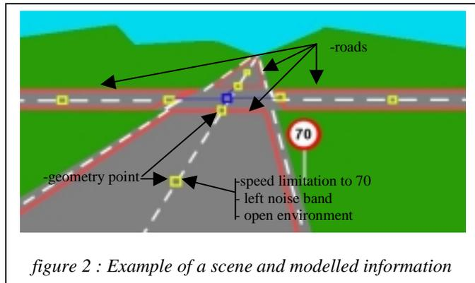
figure 2 : Example of a scene and modelled information
