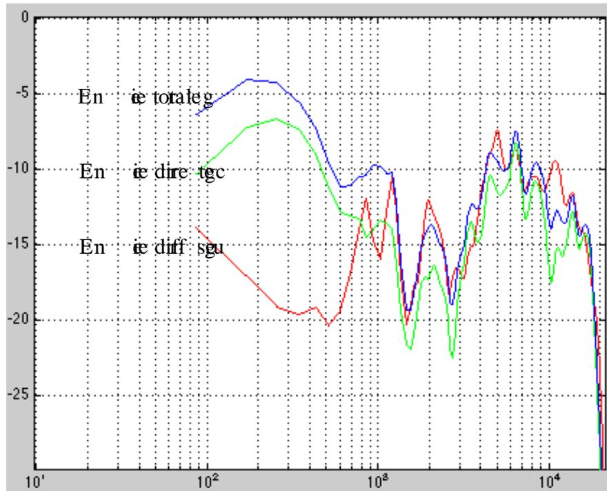
Figure 14 : spectral densities associated to the direct sound (green), to the global energy (blue) and to the diffused energy (red) after averaging the response of each loudspeakers of the cockpit
