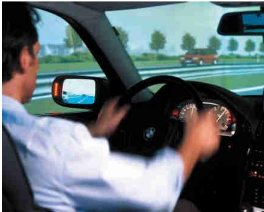
Fig. 8: Lane-change assistance warning (red light on the outside mirror)
