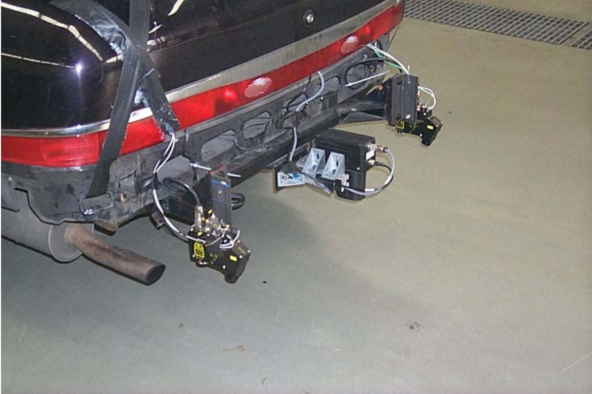
Figure 3. Laser displacement sensors, accelerometers, and non-contact speed sensor used to obtain road profiles.
