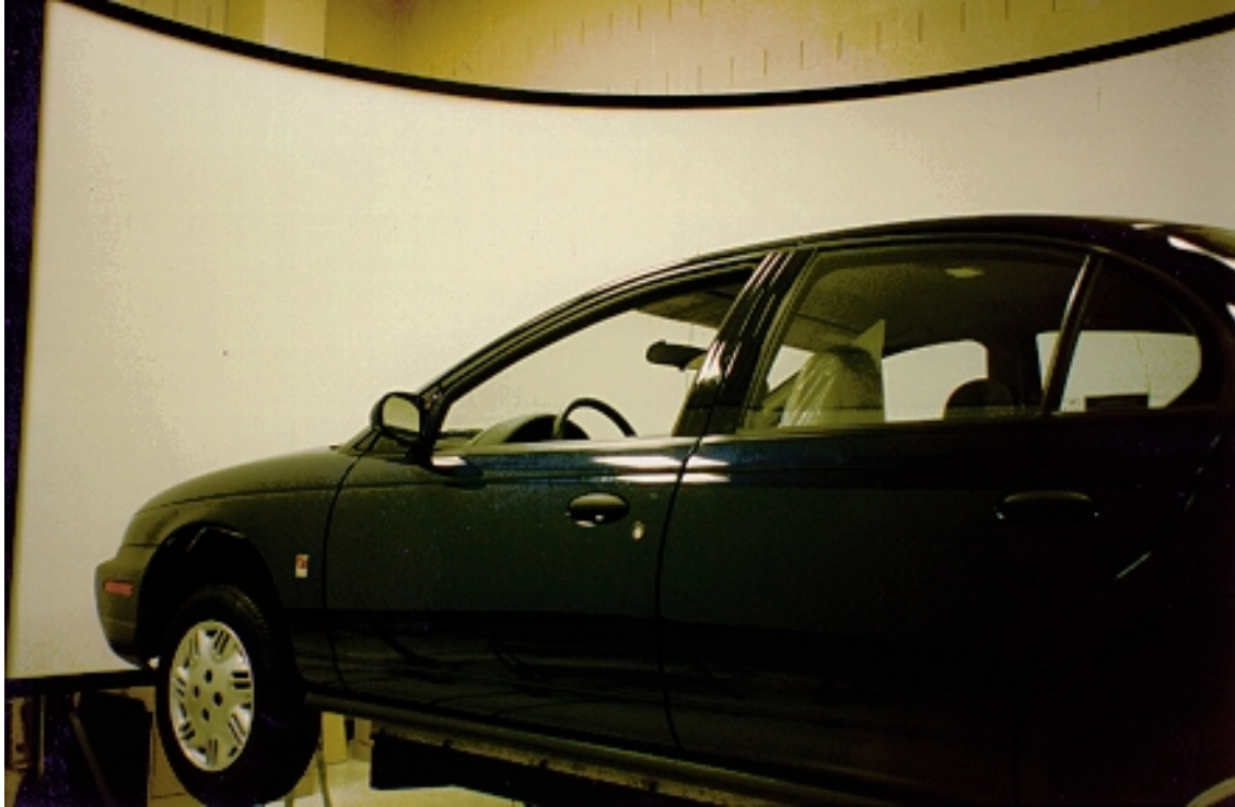
Figure 2. HYSIM car cab and cylindrical front screen.
