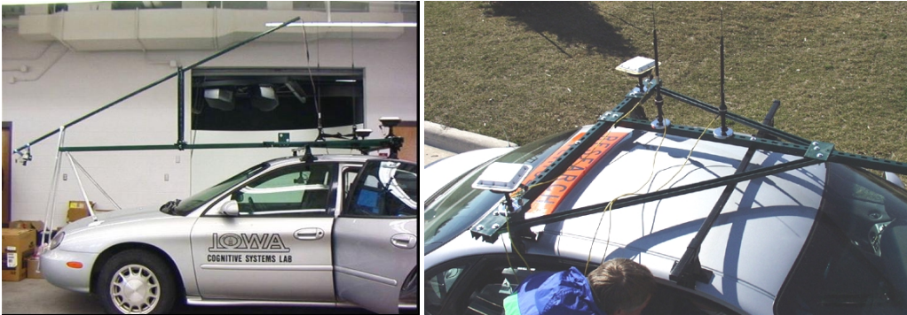
FIGURE 1 Two views of the instrumented vehicle used for the first data collection.
