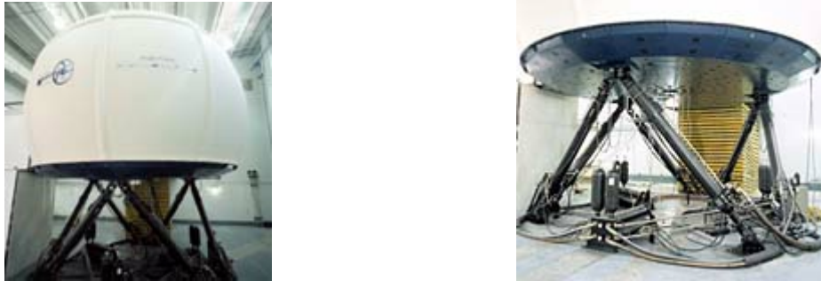
FIGURES 20a, 20b Ford VIRTEX motion base and dome.
