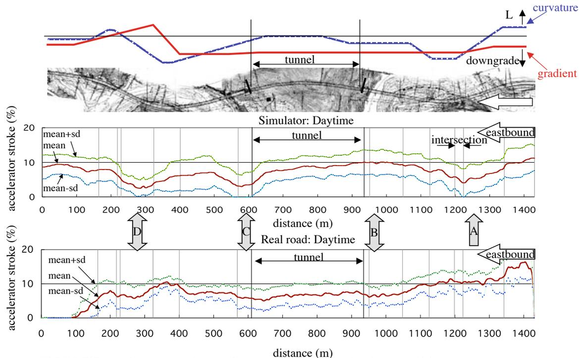
**FIGURE 7 Accelerator stroke for the eastbound trip in daytime conditions**
