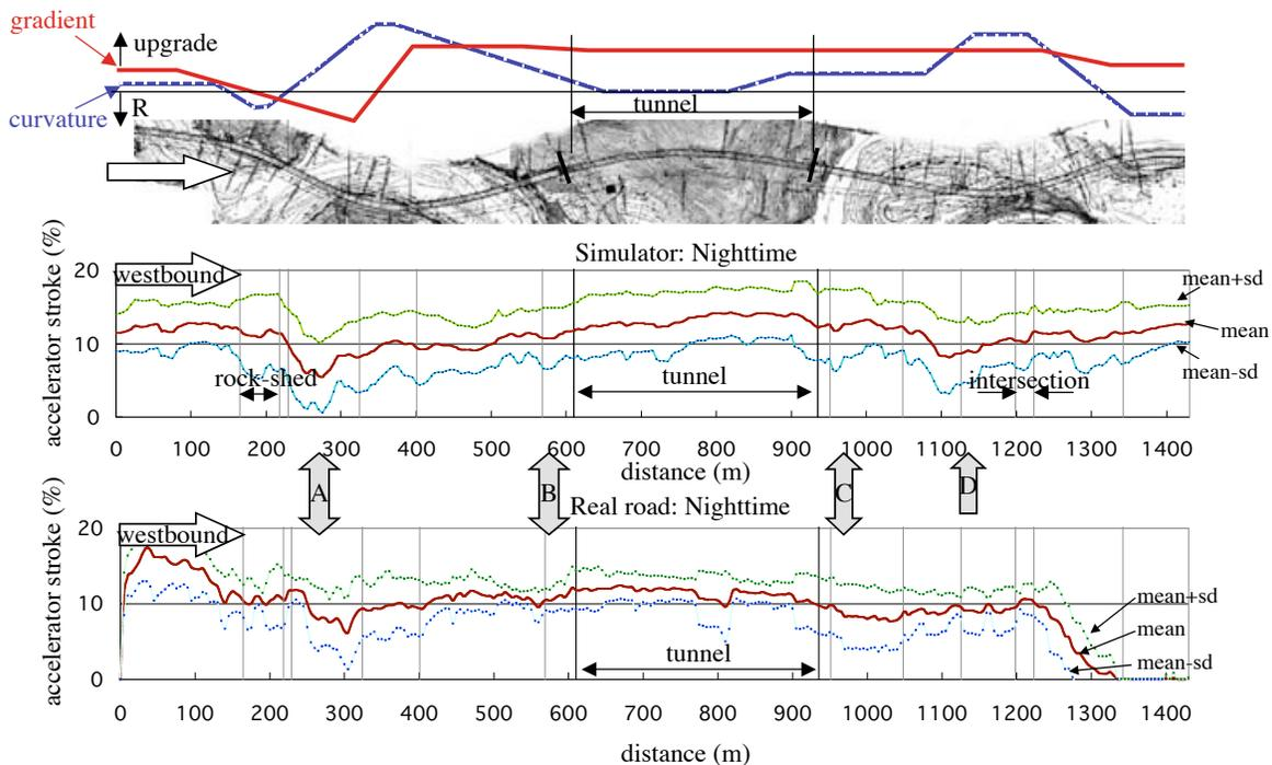
**FIGURE 8 Accelerator stroke for the westbound trip in nighttime conditions**
