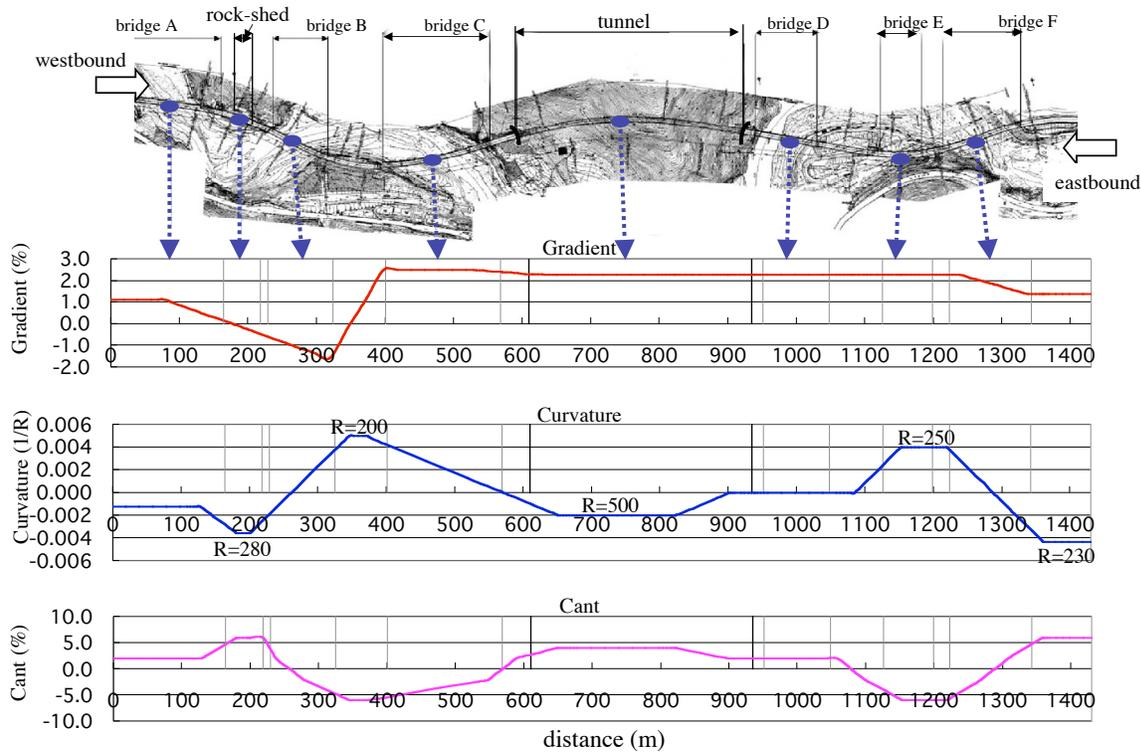
FIGURE 4 Top view, vertical profile, curvature and cant of the road section
