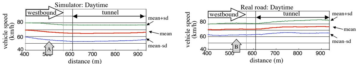
FIGURE 6 Vehicle speed before and along the the tunnel for the westbound trip in daytime conditions.
