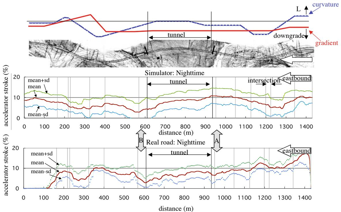
**FIGURE 9 Accelerator stroke for the eastbound trip in nighttime conditions**
