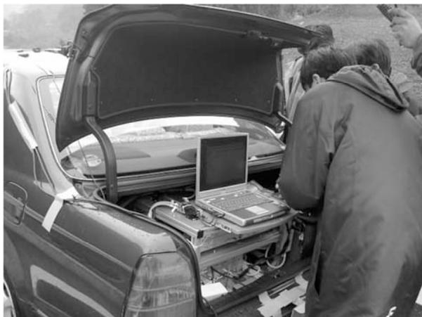
**FIGURE 3 Drive recorder system in the instrumented vehicle.**
