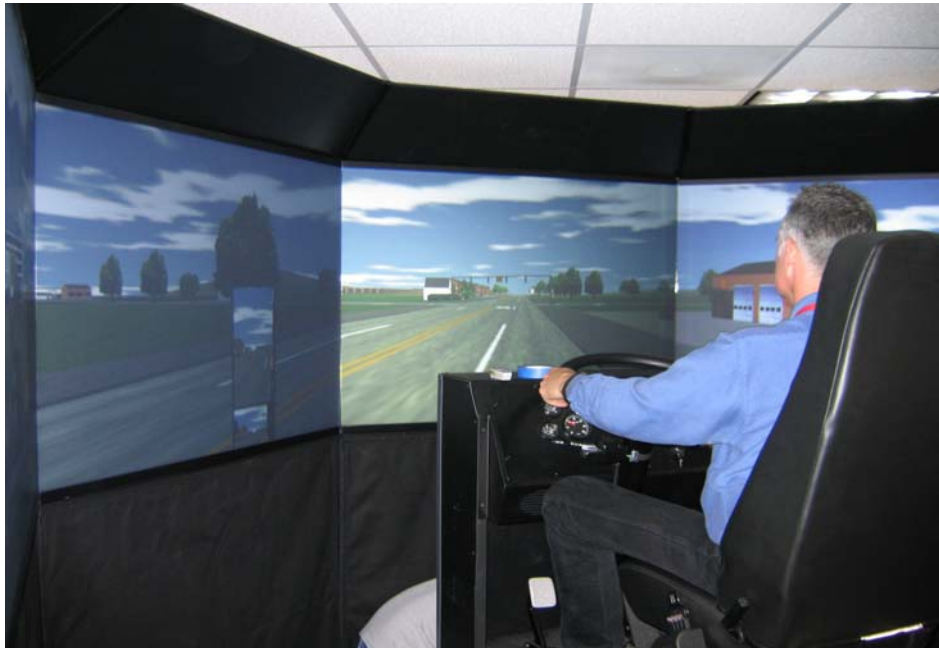
Figure 1. FAAC, Inc. TT-2000 simulator employed in the SimVal study.
