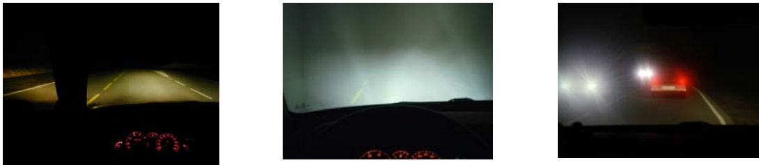
Figure 1 : headlight simulator (left), lighting simulation within fog (center), glare effects (right)
