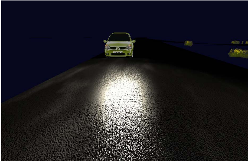
Figure 6 : rendering based on measured BRDF of wet asphalt combined with normal mapping.
