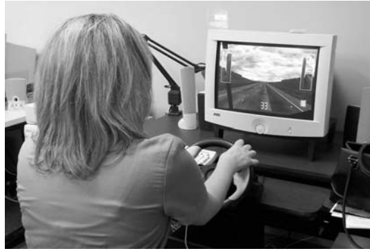
Figure 1 – Level 1 PC Driving Simulator with Joystick Steering Configuration
