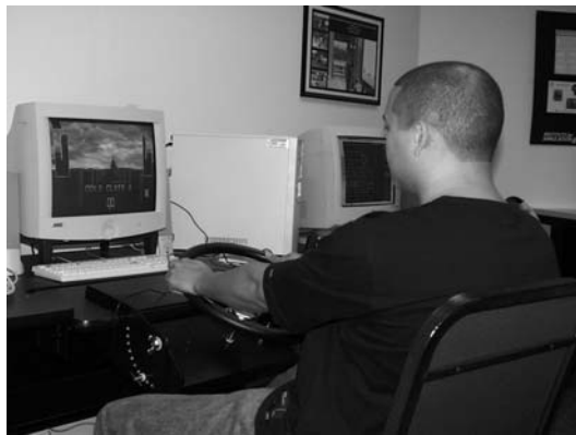
Figure 1 – Level 1 PC Driving Simulator with Joystick Steering Configuration
