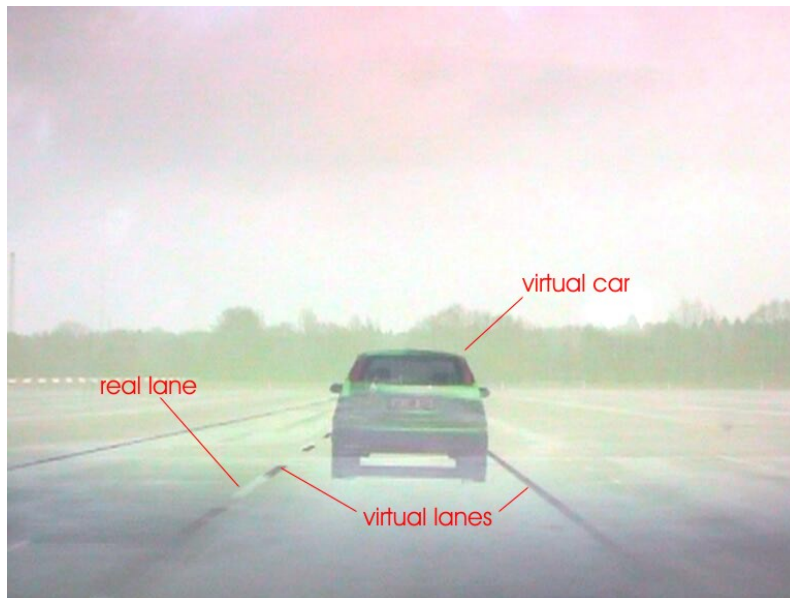
Fig. 6: Augmented reality demonstration of the Vehicle in the Loop
