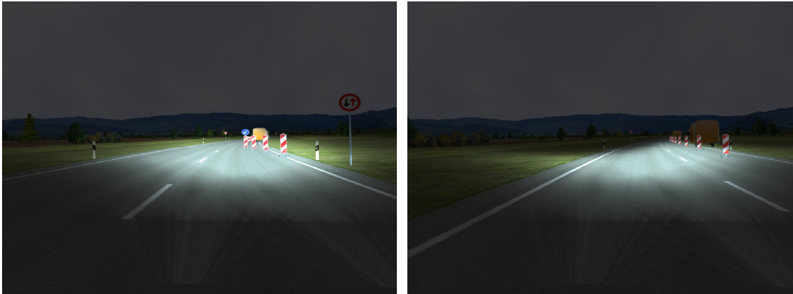
Fig. 1: Approaching a construction area with high beam (left) and low beam (right) head lights.
