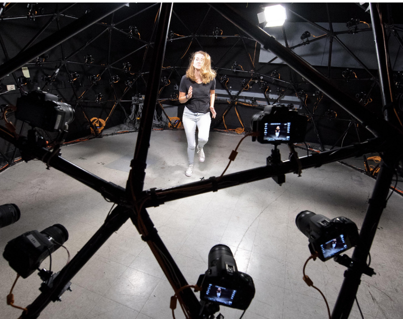
Capturing motion: A student runs in place in Dr. Stephen Baek's Visual Intelligence Laboratory's 4D scanning system. This 19-foot diameter geodesic dome structure has 100 DSLR cameras precisely synchronized and controlled via an opto-isolated control circuit developed in-house. The cameras are linked to a network of computers such that the high resolution videos recorded by the cameras are efficiently processed in parallel.
