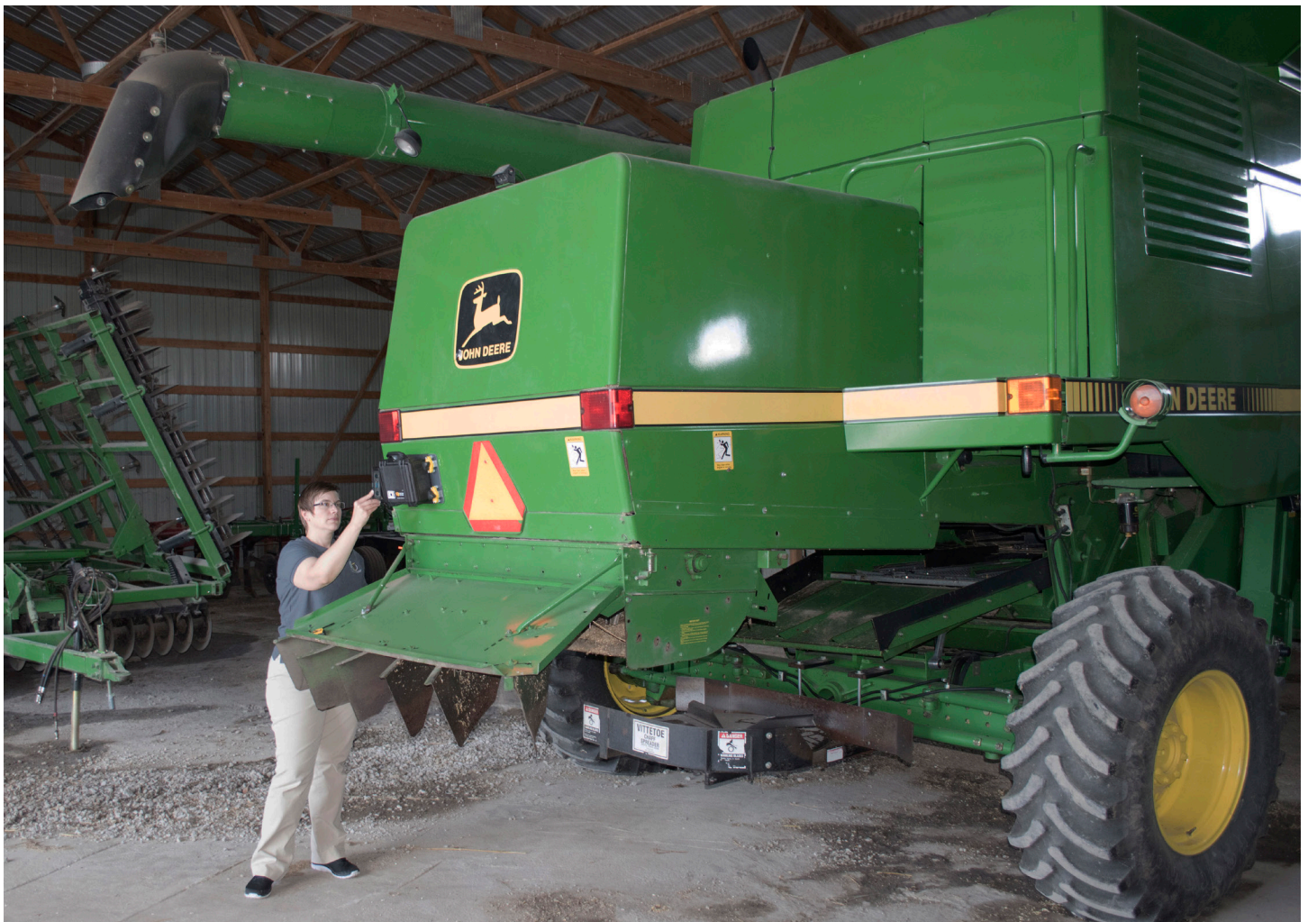
Top: SafiTrek devices prepped and ready for deployment. SafiTrek systems are attached to farm equipment using strong magnets. Bottom: Research Associate Michelle Reyes switches the magnets of a newly attached SafiTrek device on a local farmer's combine. SafiTrek devices video record vehicles as they approach, follow, and begin to pass the farm equipment.
