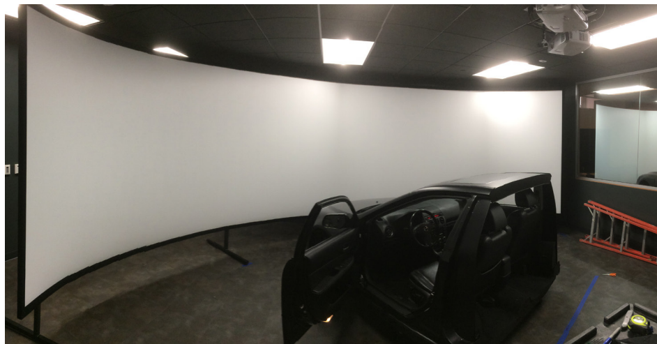
Custom half-cab miniSim with a two-projector display system built for Yale University's Developmental Neurocognitive Driving Simulation Research Center
