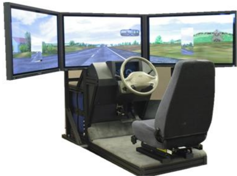
MiniSim™ driving simulator with 3 plasma display and quarter open cab setup
