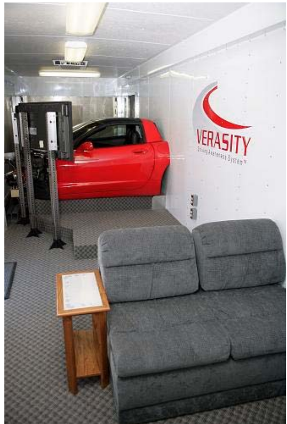
Corvette-based MiniSim™ installed in trailer installed (photo courtesy of Tom Zwica)
