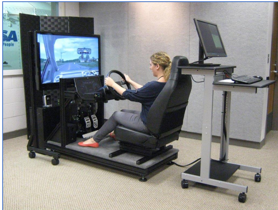
Figure 3: Simplified Cab shown with single monitor stand, 46" LCD, standing desk
