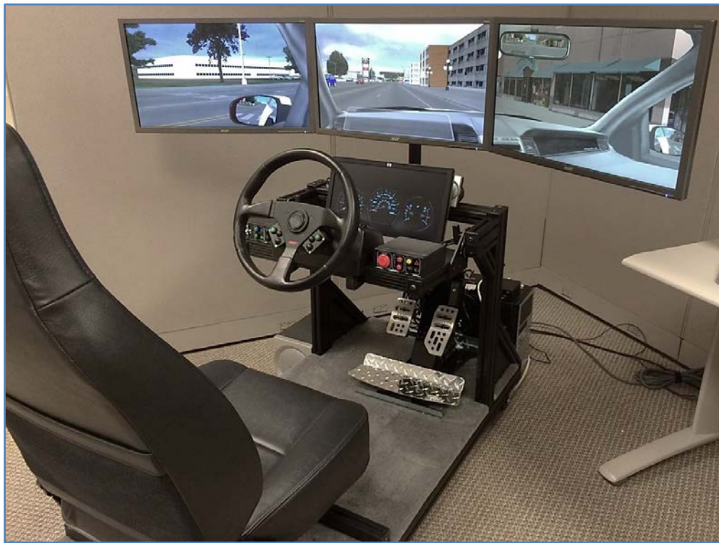
Figure 1: Simplified Cab shown with three 24-inch LCDs
