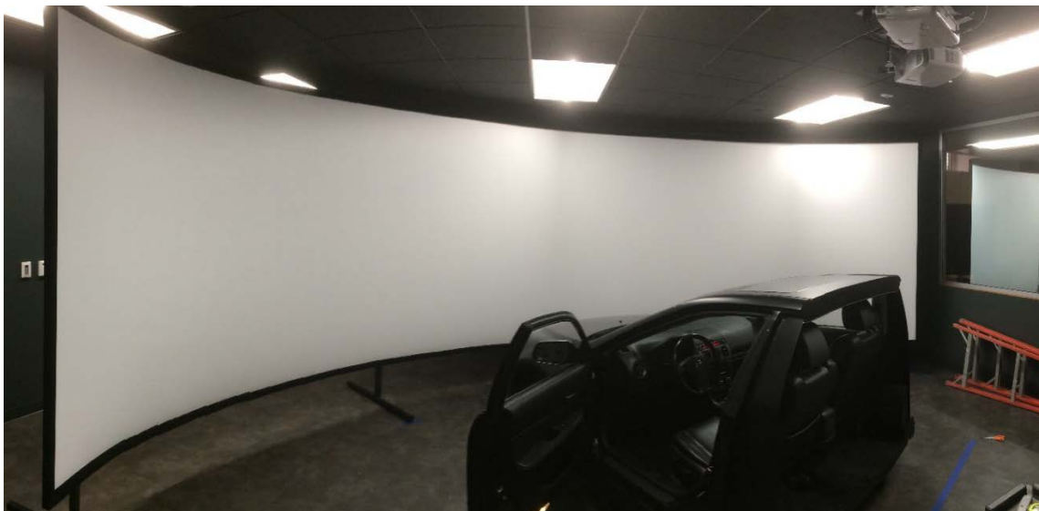
Curved Screen Installation (166-deg FOV shown)
