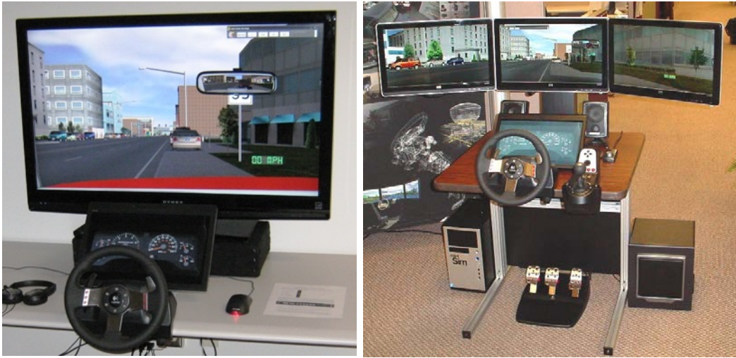
Figure 1: Desktop miniSim™ Driving Simulator with single 42" Display (L), and optional three 20" LCD Displays (R).
