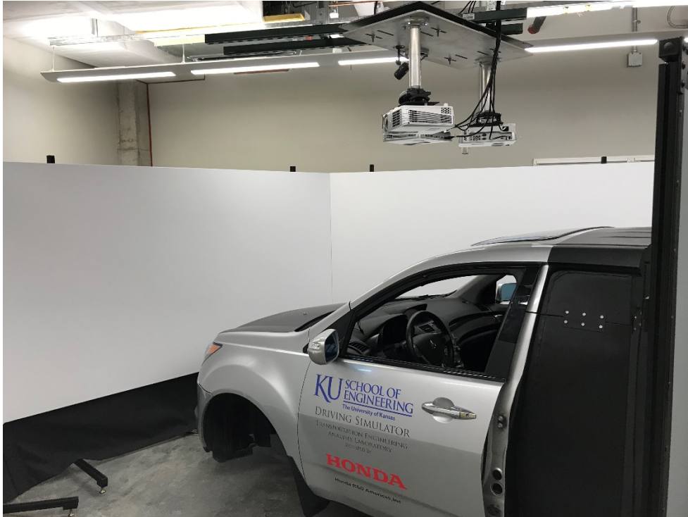
Three Flat Screens Installation (170-Deg HFOV)
