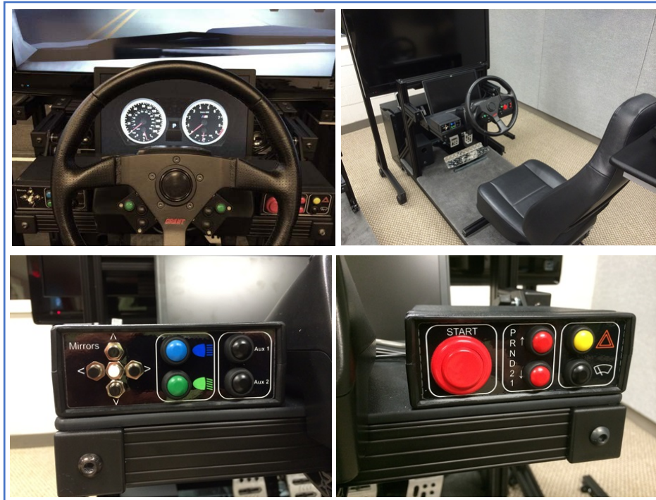
Figure 4: 13" Leather-Wrapped Wheel and Button Boxes with Labeled Buttons
