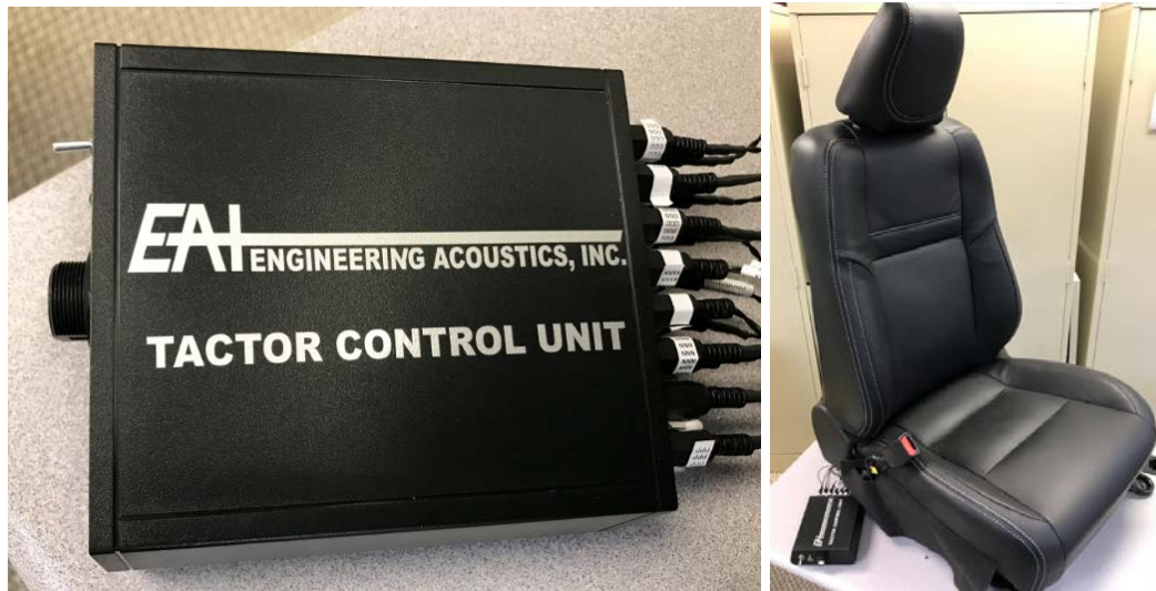
Haptic Seat Created using EAI's Tactor Control and API
