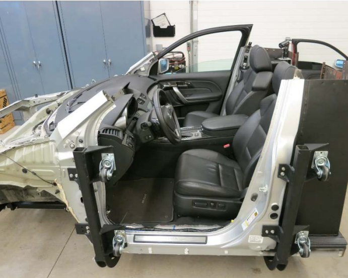
Cab Modified to Fit Doorways
