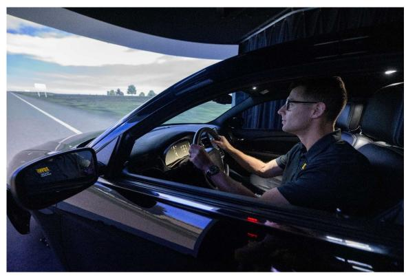
Features DSRI Infotainment and VideoCapture systems, enhanced rendering using *Unreal Engine*, steering loader from *Sensodrive GmbH*, and motion from *D-Box Technologies, Inc.*
